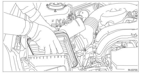
6) Remove the bolt (A) and nut (B) which secure the air cleaner case (front) to the body.
