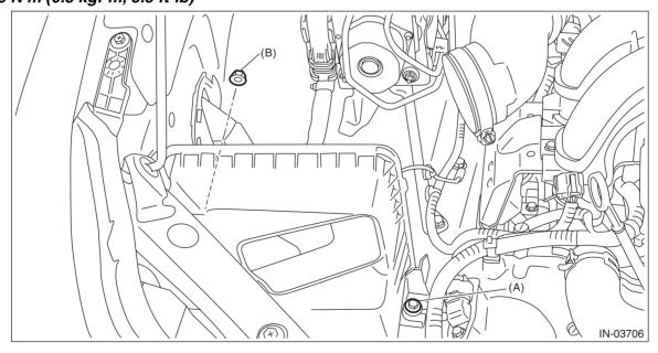
2) Install the air cleaner case (rear) and air cleaner element.
