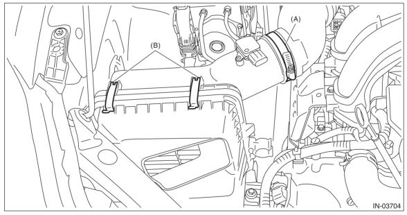
4) Connect the connector (A) to the mass air flow and intake air temperature sensor and secure the harness with clip (B).
