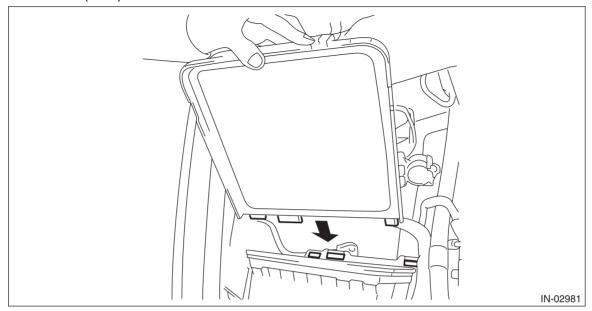
3) Install the clips (B) to the air cleaner case (front), then tighten the clamp (A) that secures the air intake boot to the air cleaner case (rear).
