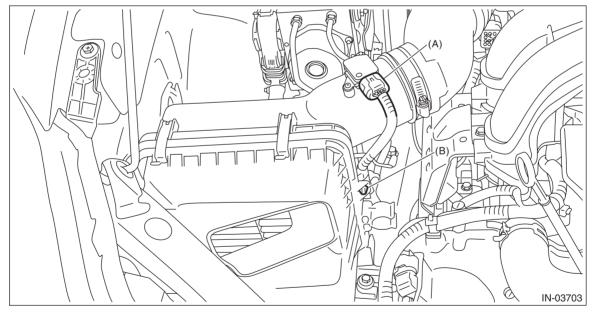
4) Loosen the clamp (A) which secures the air intake boot to the air cleaner case (rear), and then remove the clip (B) from the air cleaner case (front).
